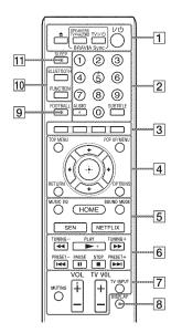
Number 5, AUDIO, VOL +, and ▶ buttons have a tactile dot. Use the tactile dot as a reference when operating the remote control.
