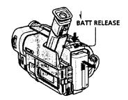
After installing the battery pack Do not carry your camcorder by holding the battery pack. If you do so, the battery pack may slide off your camcorder unintentionally, damaging your camcorder.
