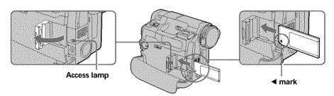
To eject the "Memory Stick," open the lid of the "Memory Stick" slot, slide MEMORY EJECT in the direction of the arrow.
