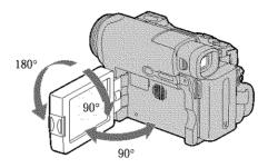
When you adjust the LCD panel, make sure that the LCD panel is opened up to 90 degrees.
