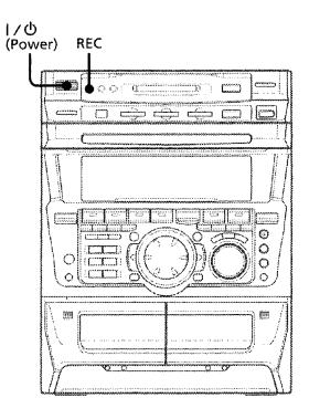
→ Press REC while recording at the point you want to add a track mark. A track mark is added that location.
