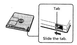
• If the MD is record protected, "C11" and "Protected" appears in the display alternately and the MD cannot be recorded on. Slide the tab to closed position, reinsert the MD and try again.
