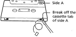
If you later want to reuse the tape for recording, cover the broken tab with adhesive tape. However, be careful not to cover the detector slots which allow the tape player to automatically detect the type of tape.
