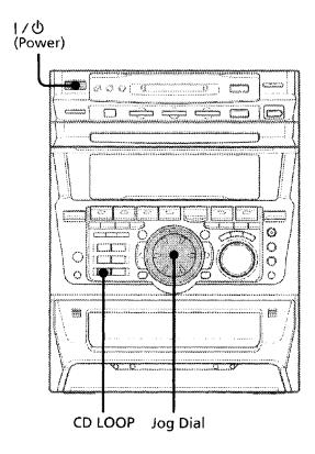
Press and hold CD LOOP during playback at the point you want to start the Loop function, and release to resume normal play.
