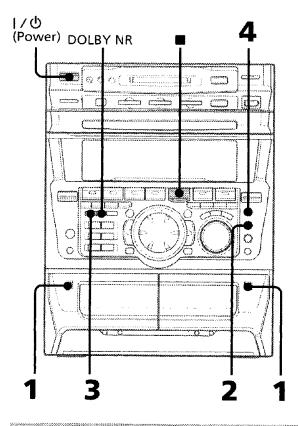
Press and insert a recorded tape in deck A and a blank tape in deck B.
