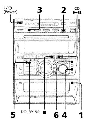
Press and insert a blank tape into deck B.
