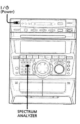
→ Press SPECTRUM ANALYZER. The display changes.
