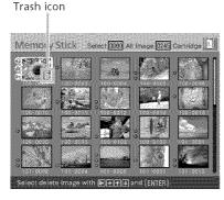
4 Press the arrow (★/★/★/♥) button to move the trash icon to the image you want to delete, then press ENTER.
