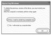
After the computer is restarted, the relevant files will be deleted and uninstallation is complete.
