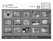
Press the arrow (\*/\*/\*/\*) button to select the desired image, then press ENTER.
