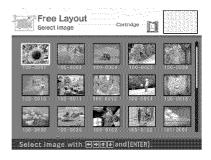
Press the arrow (\*/\*/\*/\*) button to select the desired image, then press ENTER. The window used for adjusting the image size and position is displayed.
