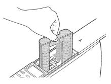
**3** Remove the paper tray from the printer. If there is print paper in the tray, remove the print paper from the tray.
