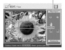
Press the arrow (\*/\*/\*/\*) button to select the desired adjustment tool, then press ENTER to adjust the size and position of the characters. To make multiple adjustments, repeat this step.
