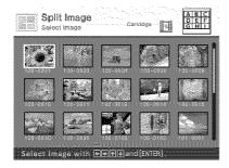
Press the arrow (\*/\*/\*/\*) button to select the desired image, and then press ENTER. The window used for adjusting the image position is displayed.
