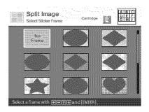
6 Press the arrow (★/★/★/♥) button to select the desired frame that you wan to add to an image, then press ENTER. If you do not want to use any frame, select "No Frame." The image list is displayed.
