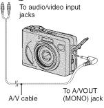
• If your TV has stereo input jacks, connect the audio plug (black) of the A/V cable to the left audio jack.
