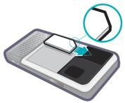
3 Insert the SIM card into the SIM. card holder. Make sure you insert it as shown in the image.
