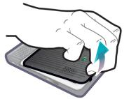
1 Open the battery cover by pressing and pulling the lower part of the cover at the bottom of the phone.
