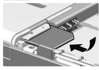
Remove the battery (if it is in place) and insert the SIM card into the SIM card holder. A PIN code is supplied with the SIM card and must be entered when switching on the phone for the first time.
