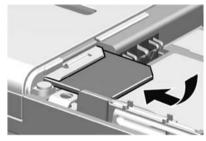
Remove the battery (if it is in place) and insert the STM card into the STM card holder. A PTN code is supplied with the SIM card and must
