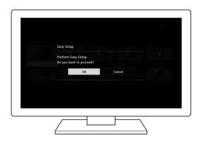
1 Press HOME on the remote control of the system. The Easy Setup screen is displayed on the TV screen. If the Easy Setup screen does not appear, use the remote control of the TV to switch the TV input setting to the HDMI IN jack that connects the TV to the system.
