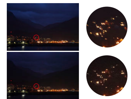
Compensation for roll shake on the Z-axis during long exposures. Most in-lens systems for interchangeable-lens cameras cannot compensate for roll shake.
