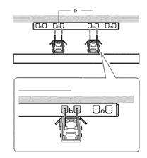
**3** Adjust the angle of the Mounting Hook.
