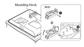
**4** Align the holes on the right Mounting Hook with the corresponding holes on the rear of the TV.
