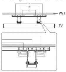
**3** Adjust the angle of the Mounting Hook.
