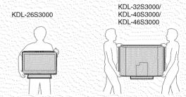
☐ When lifting or moving the TV, hold it firmly from the bottom. Place your palm directly under the panel.
