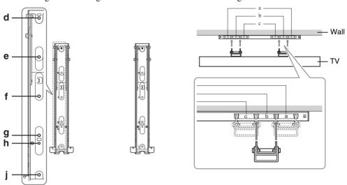
2 Adjust the angle of the Mounting Hook.
