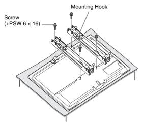
**3** Be sure to tighten the screws with equal torque strength.
