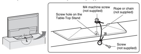
The length of the M4 machine screw differs depending on the rope or chain diameter. Please refer to right illustration.
