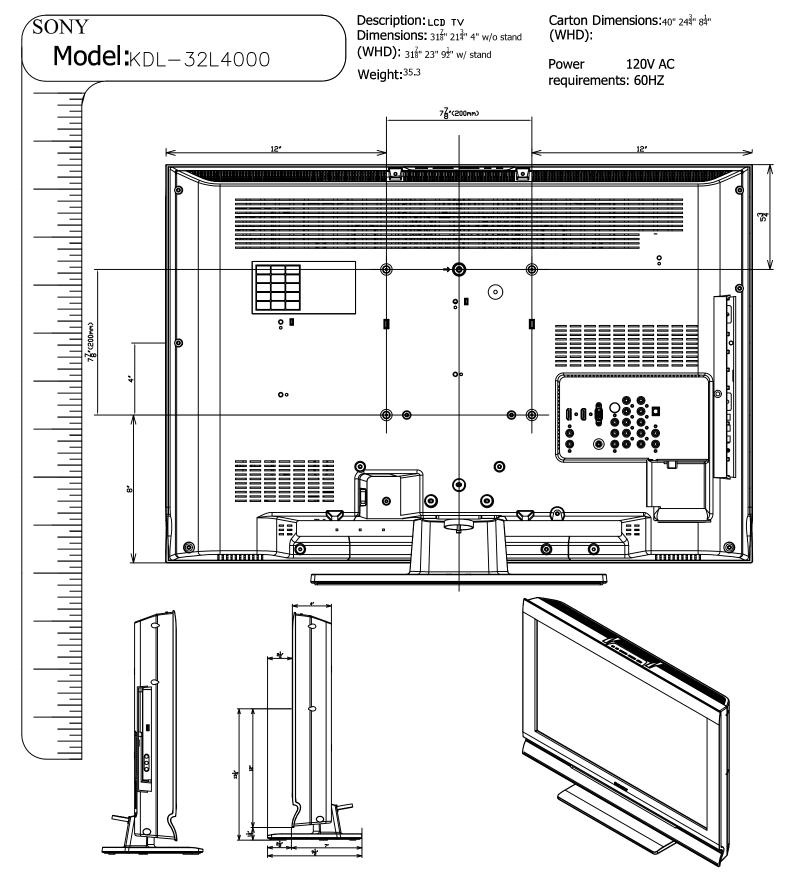
NOTE: WHERE THERE ARE CLOSE TOLERANCES INVOLVED IN CABINET BUILDING OR APPLICATIONS WHICH REQUIRE A GREAT DEGREE OF PRECISION, WE RECOMMEND THAT THE PRODUCT ITSLEF BE USED TO MAKE THE ACTUAL MEASUREMENTS. SONY WILL NOT BE HELD RESPONSIBLE FOR INACURRACIES IN THE DESIGN OR MANUFACTURE OF ENCLOSURES.
