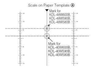
4 Tape the Paper Template (a) to the wall and drill holes according to the numbering on the Paper Template (a) using an electric drill.
