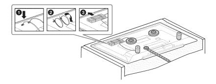
10 Install the TV on the wall. Confirm the Pulleys © are firmly latched into the Wall-Mount Base ®. Then, attach the Band 🕞 to the wall using a screw (5 mm in diameter, not supplied).
