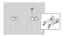
Attach the Pulleys © to the TV using the supplied screws Φ. Attach the Spacers E to the holes indicated by the triangle marks Δ. Then, attach the Band F using the supplied screw Φ.
