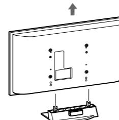
**3 Attach the supplied four hooks on the rear side of the TV.**
