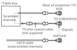
For this set up, you can switch between scrambled channels (through your cable box), and normal (CATV) channels by pressing ANT on your remote control.
