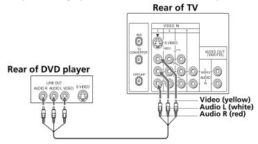
For optimum picture quality, use S VIDEO instead of the yellow Audio/ Video cable. S VIDEO does not provide sound, the audio cables must still be connected.
