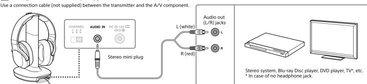
If the sound is distorted by connecting the transmitter to the A/V component's audio out (L/R) jacks, reconnect the transmitter to the headphone jack.
