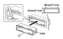
**2** Mount the unit onto the bracket ①, then attach the protection collar ③.
