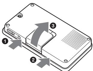
**4 Remove the battery.**
