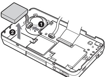
**5 Insulate the connector terminal by wrapping with a tape.****Notes on the lithium-ion battery**
