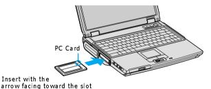
2 Push the PC Card gently into the slot. The PC Card is automatically detected by your system. The Unplug or Eject Hardware icon appears in the taskbar.
