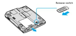
If you do not plan to install another device into the multipurpose bay, insert the supplied weigh saver to protect the bay.
