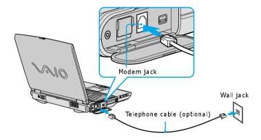
2 Plug the other end of the telephone cable into the wall jack.
