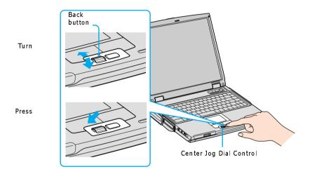
The center Jog Dial Control window always appears in the display. It is either in the launcher mode or in the guide mode.
