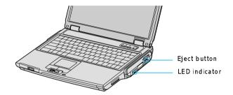
2 Push the Eject button, and remove the disk.
