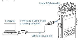
2 Make sure that your linear PCM recorder is recognized correctly by your computer.
