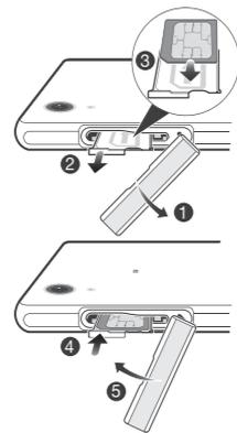
! Inserting the micro SIM card into the device without the SIM card holder could damage your micro SIM card or your device, and Sony Mobile does not warrant and will not be responsible for any damage caused by such action.
