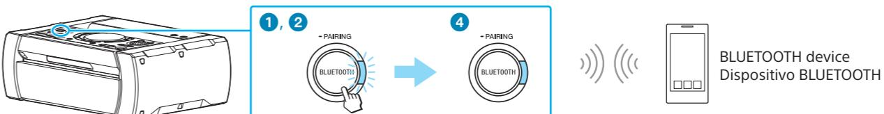
Be sure to place the BLUETOOTH device within 1 meter (3.3 feet) from the unit.
