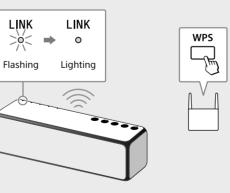
Depending on the wireless router, press and hold the Wi-Fi Protected Setup (WPS) button for a few seconds. For details, refer to the operating instructions of your router. When the LINK indicator lights up in orange, the Wi-Fi network connection is complete.
