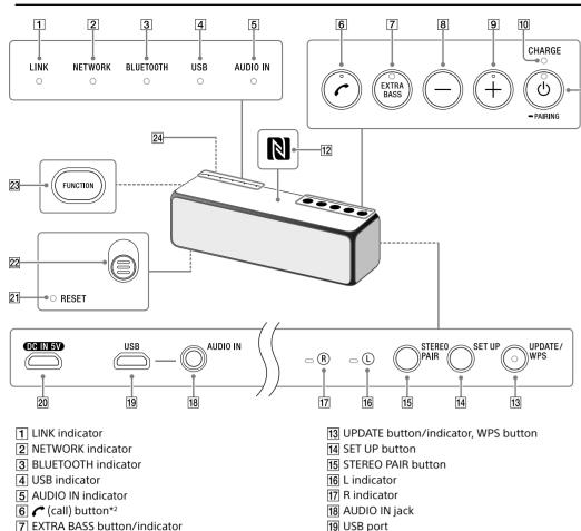
19 USB port 20 DC IN 5V jack\* 21 RESET button 22 Grille detachment leve 11 (power)/- PAIRING button/indicator **23** FUNCTION button 24 Microphone
