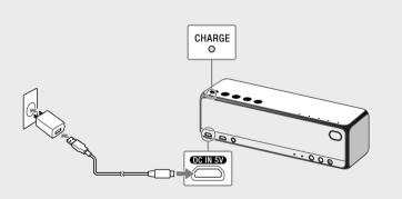
To charge the battery, connect the unit to an AC outlet by using the supplied USB AC adaptor and micro USB cable.
