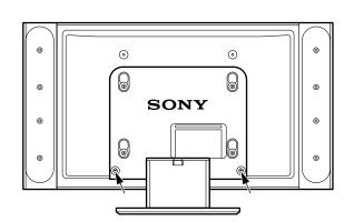
Remove the two fixing screws at the bottom of the plate as shown in the diagram.
