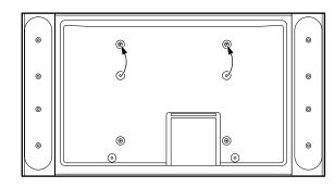
Remove the two fixing screws from the two lower holes near the upper portion of the Mounting Hook Unit, and then re-insert and tighten them in the two upper holes as shown in the diagram.
