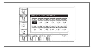
**2** Carry out the source track selection for the digital audio output signal on each channel.
