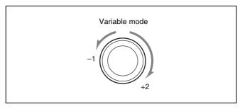
The tape is played back at a speed that corresponds to the angle of the search dial. A direction indicator (◀ or ►) lights up to indicate the direction of playback. The search dial clicks at the positions for still-picture and normal-speed playback.
