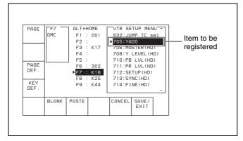
**6** Press the F7 (PASTE) button to register the item. The new item is registered to the function button.
