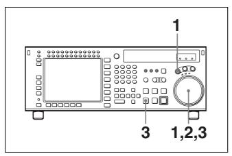
**1** Press the SHUTTLE button, turning it on. The VTR enters still-picture mode.
