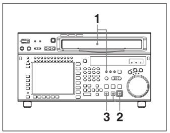
1 Check that the REC INHIBIT indicator is off, then insert a cassette.
