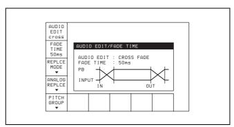
**2** Press the ALT/F2 (FADE TIME) button to select the fade time.
