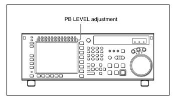
You can also carry out the playing level adjustment using the VTR SETUP menu item 833 "AUDIO PB LEVEL".
