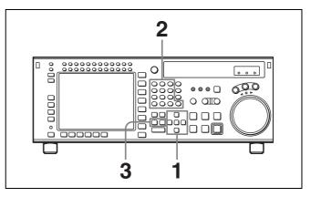
Use the cursor buttons to move the cursor to the IN/ OUT section to be entered or modified.
