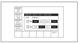
2 Use the F1 (ANAREP CH9), F2 (ANAREP CH10), F3 (ANAREP CH11), F4 (ANAREP CH12) buttons to specify whether to control channels 9 to 12 with edit preset commands for analog channels 1 and 2.
