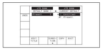
The procedure for saving from CURRENT DEFAULT to DEFAULT BANK, saving from DEFAULT BANK or FACTORY PRESET (factory setting) to CURRENT DEFAULT, changing the title, or setting protection, is the same as operation on a VTR bank.
