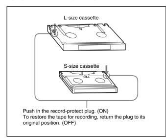
When a cassette with this plug pushed in is inserted into the VTR, the REC INHIBIT indicator on the lower control panel lights up and recording will not start, even if you press the REC/EDIT button.
