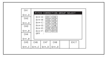
**2** Use the F1 (CH1) to F8 (CH8) buttons and the ALT/F1 (CH9) to ALT/F4 (CH12) buttons to group channels (Group-A to F, OFF).
