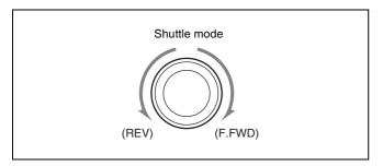
The tape is played back at a speed that corresponds to the angle of the search dial. A direction indicator ( $\triangleleft$  or  $\blacktriangleright$ ) lights up to indicate the direction of playback. The search dial clicks at the positions for still-picture and  $\pm 10$  times normal-speed playback.
