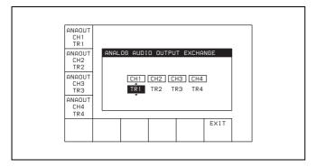
**2** Carry out the source track selection for the analog audio output signal on each channel.
