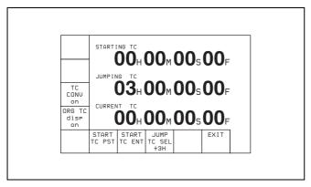
**STARTING TC:** Time code used as a reference when converting time code.
