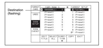
The flashing cursor bar indicates the storage destination.
