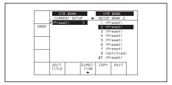
**3** Press the F8 (DIRECTION) button to select the ← direction.
