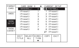
3 Press the F8 (DIRECTION) button to select the ← direction.
