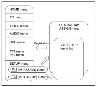
PF button assignment allows you to assign the same item also to a different menu screen or button.
