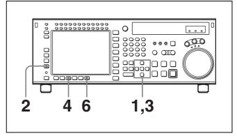
**1** Press the cursor buttons to move the cursor to the cut data to be changed.
