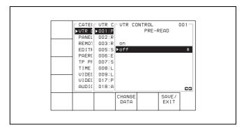
4 With the F8 (CHANGE DATA) button, or the cursor ↑ and ↓ button, or the MULTI CONTROL knob, select the setting value.
