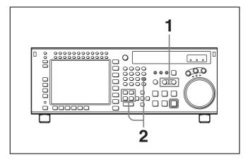
1 Press the RECORDER or PLAYER button to select the VTR on which to perform the edit point deletion.
