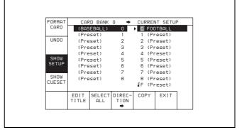
**3** Press the F8 (DIRECTION) button to select the → direction.
