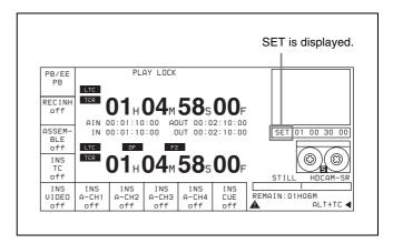
**5** Press any of the IN, OUT, AUDIO IN, and AUDIO OUT buttons.
