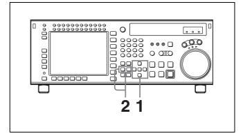
1 Use the cursor buttons to move the cursor to the IN/OUT section on which the current log data is to be entered or modified.
