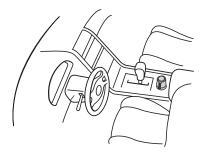
2 Secure the rotary commander to the flat place by pressing the Velcro tapes firmly together.
