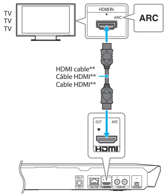
\* The ARC function enables the TV to transfer audio back to this system via a single HDMI cable. To check the compatibility of your TV's ARC function, refer to the operating instructions supplied with your TV.
