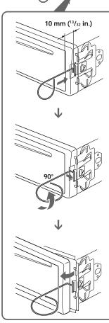
2 Insert a flathead screwdriver between the bracket and mounting spring. Gently pry the spring toward the unit while pulling the unit out a little. Repeat on the opposite side and remove the unit.
