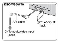
If your TV has stereo input jacks, connect the audio plug (black) of the cable for multi-use terminal (DSC-W50/W70) or the A/V cable (DSC-W30/W40) to the left audio jack.
