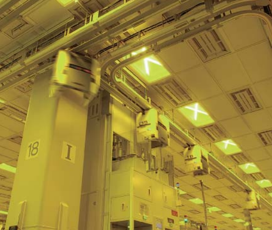
The automated material handling system installed to new 300mm wafer line
