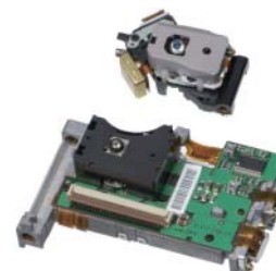
Optical pickup for conventional DVDs/CDs (top) and Blu-ray Disc (bottom)
