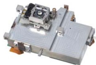
Prototype of the newly developed three-wavelength optical pickup for recording and playback
