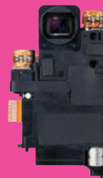
Newly designed folded-optics lens system
