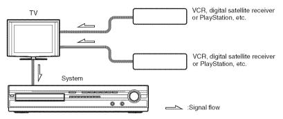
Select the component on the TV. For details, refer to the operating instructions of the TV. If the TV does not have multiple audio/video inputs, a switcher will be necessary to receive the sound from more than two components.
