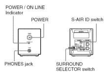
The unit transmits sound to the surround amplifier that is connected to the surround speakers. To establish sound transmission, perform the following Steps.
