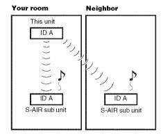
After pairing, sound transmission is established between the paired unit and S-AIR sub unit(s) only.
