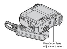
Adjust the viewfinder lens adjustment lever until the picture is clear.
