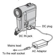
You can charge the battery pack on a trip, even if you have not brought the Handycam Station along. With the ▲ mark on the DC plug facing front, connect the AC Adaptor to the DC IN jack on your camcorder as shown in the illustration.
