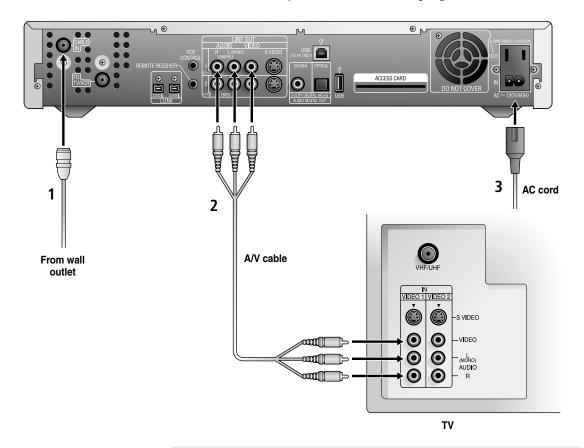
If your TV has an S VIDEO jack: For best picture quality, use an S VIDEO connection instead of the yellow video cable on your combined A/V cable. Using an S VIDEO cable, connect the Digital Network Receiver's S VIDEO OUT jack to the TV's S VIDEO IN jack. S VIDEO does not provide audio, so audio cables must still be connected to provide sound.
