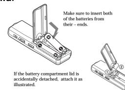
Clock setting display appears when you insert batteries for the first time, or when you replace the batteries with new ones. Please refer to Steps 2 to 3 in "Step 2: Setting the Clock" to set the date and time
