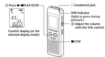
After playing back one message, the unit stops at the beginning of the next message. When the continuous play function is set to "ON" (see the reverse side), the unit stops after playing all messages in a folder. When the last message on a folder has been played back, the unit stops at the
