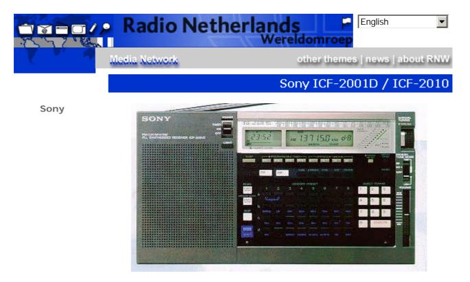
Year Introduced/discontinued: 1985/2003 Power: 4.5 Volts DC for the radio (D size, plus 3 penlights to back-up computer and clock). AC Mains adaptor often included in the price Size: 290 x 160 x 50 mm Weight: 1800 g Price: US\$350, CAN\$500 Coverage: FM, LW, MW, SW (150 - 29999 kHz) & 116-136 MHz
