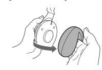
2 Place the new ear pad on the driver unit. Hang the edge of the ear pad on one side of the driver unit's groove edge, then turn the edge of ear pad around the driver unit as illustrated
