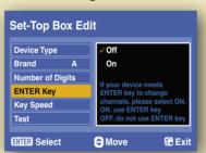
[Key Speed]: Selects the speed to send commands to the cable box/satellite receiver.
