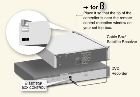
You can have the recorder control channels on the cable box or satellite receiver for timer recording. Connect the Set Top Box controller (supplied), and select "On" in step 5 of "Set top box settings" on the next page.
