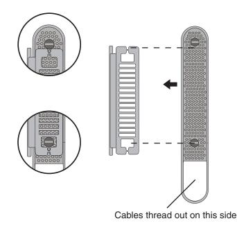
**5** Push down the receiver so both Mounting Knobs are locked into the grooves, then fully tighten the Mounting Knobs by hand.
