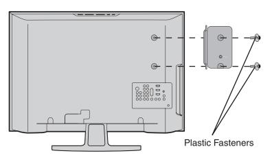
**2** Insert the 2 Plastic Fasteners (supplied) into the holes, then press in the head of the fasteners using your finger until they click.
