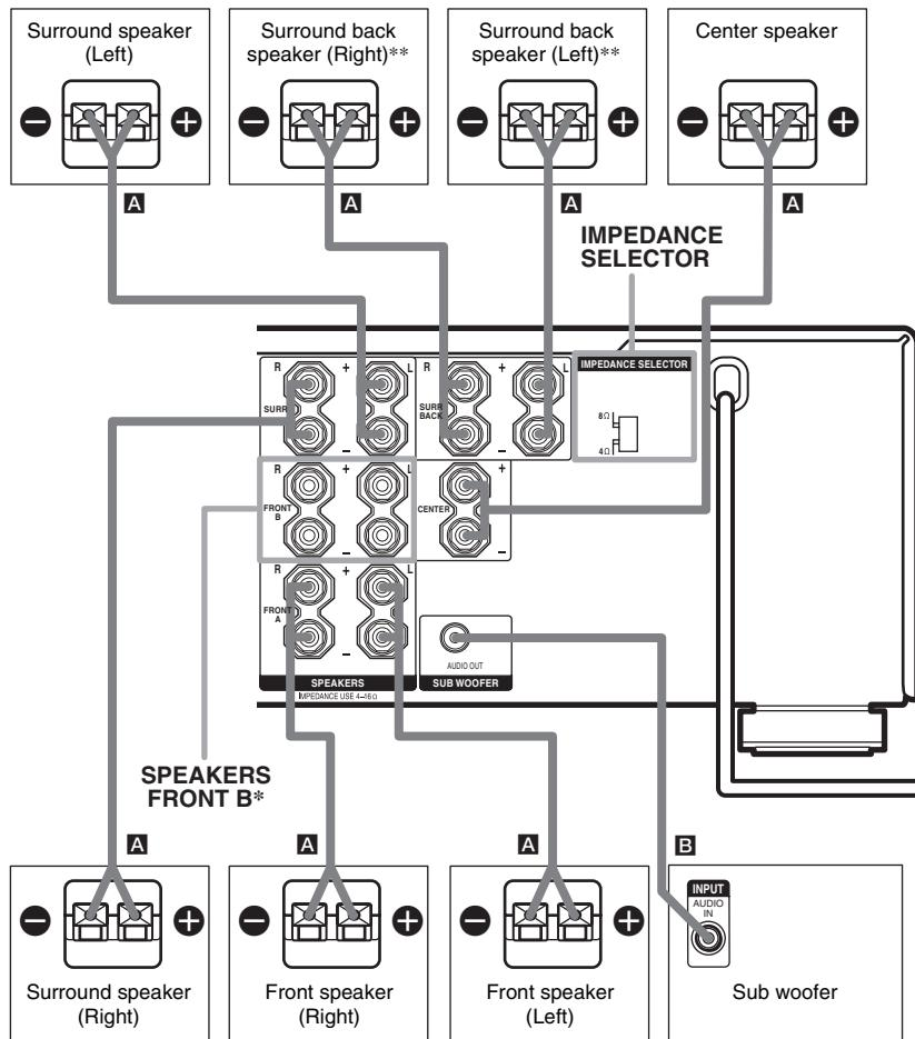
\* If you have an additional front speaker system, connect them to the SPEAKERS FRONT B terminals. You can select the front speakers you want to use with SPEAKERS (OFF/A/B/A+B) button. For details, see "Selecting the speaker system" (page 42).
