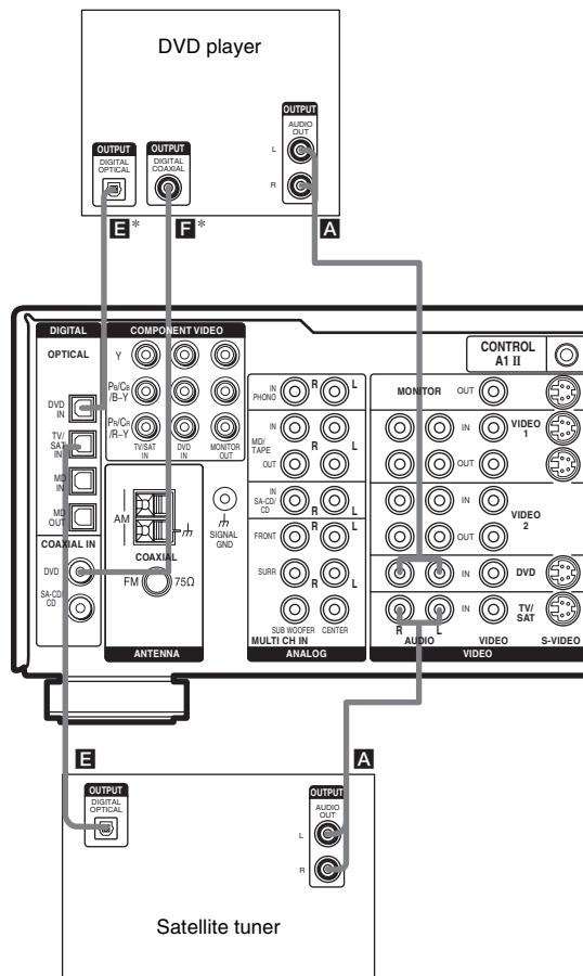
\* Connect to either the COAXIAL DVD IN or the OPTICAL DVD IN jack. We recommend making connections to the COAXIAL DVD IN jack.
