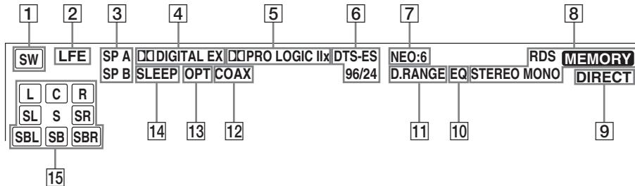
**1 SW:** Lights up when sub woofer selection is set to “YES” (page 17). While this indicator lights up, the receiver outputs the LFE signal recorded on the disc or generates a low frequency signal for output to the sub woofer. This indicator does not light during the 2CH STEREO mode.
