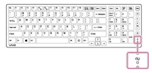
It blinks when the battery is running out of power.
