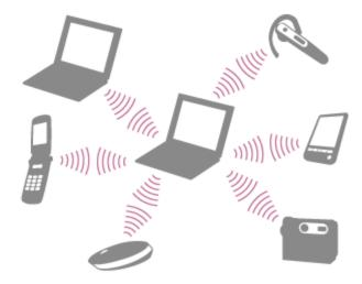
One BLUETOOTH device can connect with up to seven devices via wireless network to exchange data. When a device requires connection to another device, it sends out an inquiry to neighboring BLUETOOTH devices. If any device responds to the inquiry, the two devices can connect with each other.
