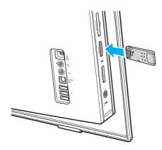
Be sure to hold the Memory Stick media with the arrow pointing in the correct direction as you insert it into the slot. To avoid damaging your computer or the Memory Stick media, do not force the Memory Stick media into the slot if you cannot insert it smoothly.
