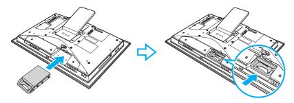
Be sure to connect the Serial ATA power cable and the Serial ATA cable.
