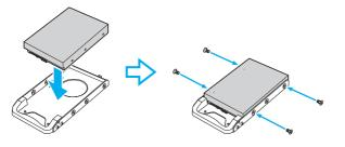
Å new hard disk drive comes with the necessary screws. Do not overtighten these screws when securing the drive to the drive holder.
