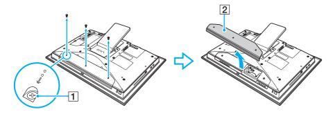
**6** Unscrew the three screws (3) securing the drive holder.
