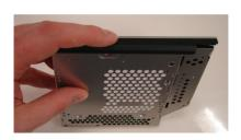
**Step 13.** Align the tabs on the bezel with the tab holes located on the ODD. Carefully press the bezel into place.
