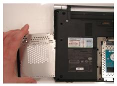
**Step 8.** Carefully remove the ODD from the unit.
