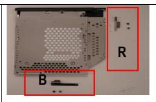
**Step 14.** Position the new ODD (Label side down) and identify the correct bracket with the correct side to be secured. Notice the different shape of each bracket and the alignment of the Bracket and ODD screw holes.
