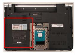
**Step 5.** Locate the Optical Disk Drive (ODD) Bay.
