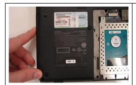
**Step 17.** Ensure that the new ODD is seated flush on the edge of the computer.
