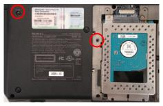
**Step 18.** Reinstall the two (2) ODD Bay screws to secure the ODD.
