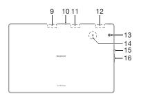
1. Headset jack 9. GPS antenna 2. Nano SIM/Memory 10. Microphone card slot cover 11.Wi-Fi sub antenna 12. Bluetooth/Main Wi-Fi Light sensor Front camera lens antenna 5. Charging/Notification 13. Main camera lens 14. NFC<sup>™</sup> detection area 6. Charger/USB port 15. Power kev 7. Speaker 16. Volume/Zoom key 8. Speaker
