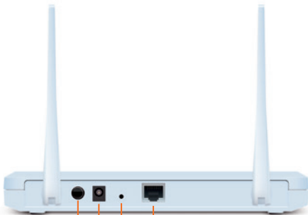
10/100/1000 Base-TX Reset Power Power on/off switch
