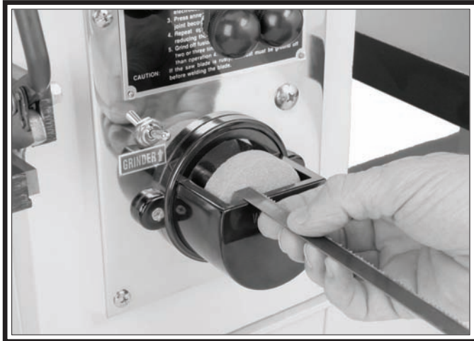
Figure 25. Using the grinder to square up the blade end.
