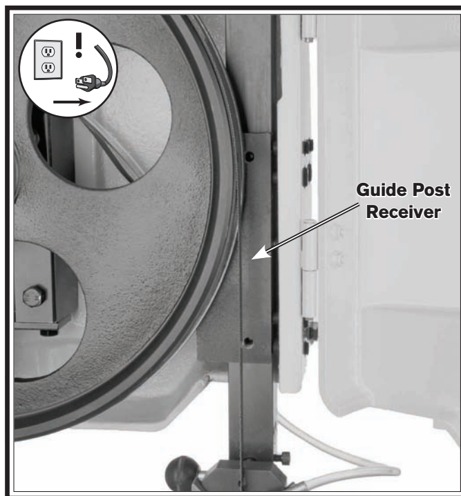
Figure 42. Guide post system.
