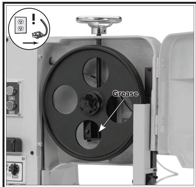
Figure 34. Upper wheel leadscrew lubrication.
