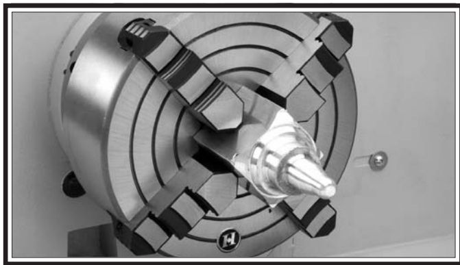
Figure 61. Example of non-concentric workpiece correctly mounted on the 4-jaw chuck.
