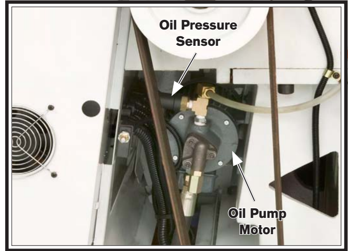
Figure 166. SB1016 Oil pump motor & pressure sensor location.
