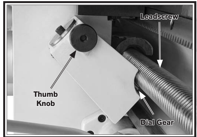
Figure 95. Thread dial gear engaged with the leadscrew.
