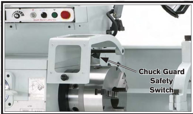
Figure 174. Chuck guard limit switch.
