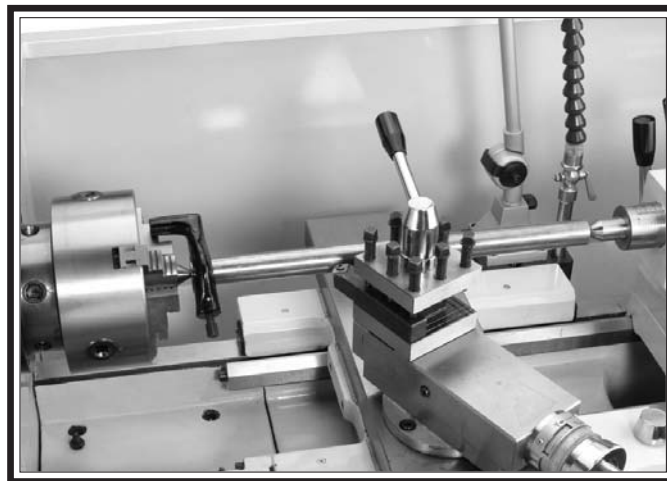
Figure 69. Example of round stock mounted between the centers.
